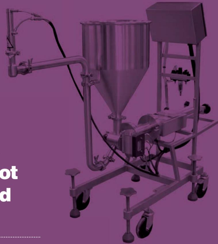
Our high quality Series Five is predominantly supplied as a fully automatic in-line depositor for use with a conveyor. It is also available as a semi-automatic unit with foot pedal operation.
